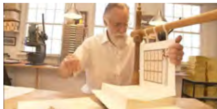
Sewing the signatures by hand to form the inner spine of the Haggadah.
